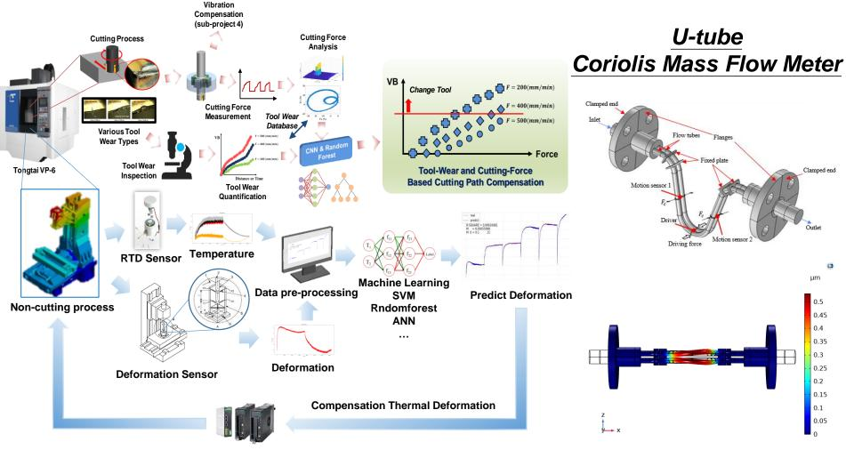
Thermal Deformation Model of CNC Using ML
